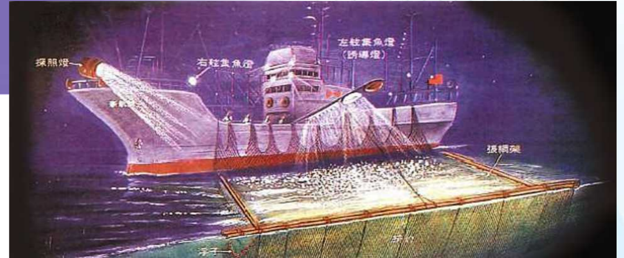
秋刀魚棒受網作業模式(左舷作業) Model of Saury net's operating (left side)
